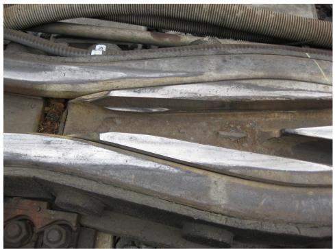
Figure 7: Observed Wing Rail Wear
