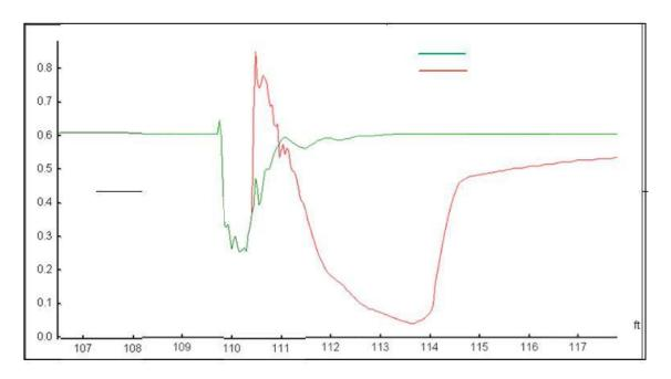
Figure 3. Comparison of L/V Ratio on the Lead Right Wheel through a Standard Frog (Green) and Expo Frog (Red)
